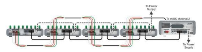
If you wish to make your own analogue link cables, use a screened cable with low dielectric loss insulation such as PTFE or polyethylene (otherwise measurement performance may be affected). The screen should be connected to the ground terminals on both millisKanners.
