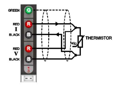
Because the resistance of thermistors used for temperature measurement is much higher than for PRTs, lead resistance is not normally a problem.
