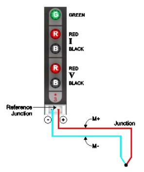
This technique is less accurate than using an ice-point or external compensation due to the additional uncertainties associated with the internal reference junction sensor and any temperature gradients between the reference junction formed within each miniature thermocouple connector and the temperature of the reference junction temperature sensor.
