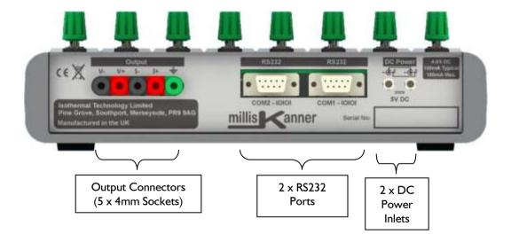
The binding posts accept 4mm plugs, spades or bare wires. The current (I) and voltage sense (V) terminals are spaced on 19mm ( $\frac{3}{4}$ ") centres so that standard BNC to 4mm adaptors (not supplied) can be used to connect to thermometer sensors that have BNC terminations
