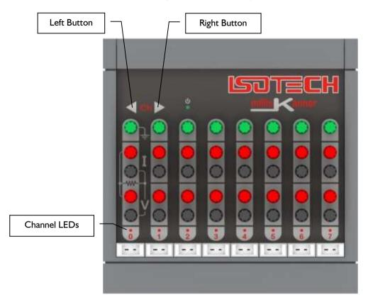
The millisKanner starts up with no channel selected. Pressing the 'Right' button will then select Channel 0. Press the 'Right' button when Channel 7 is selected or the 'Left' button when Channel 0 is selected to turn off all channels. The 'Channel LEDs' indicate which channel is selected.
