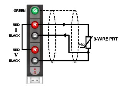
The connection between the positive (red) terminals should carry no current and should be connected as close to the base of the I+ terminal as possible in order for the 3-wire compensation to work effectively. The lowest 3-wire compensation error is achieved by using a wire under the screw terminal to connect the positive terminal together and then adding the 'single' PRT lead to the binding post:
