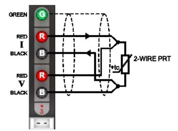
The top (green) terminal should be connected to the screen of the PRT's lead (where present) to minimise electrical noise picked up by the wires.
