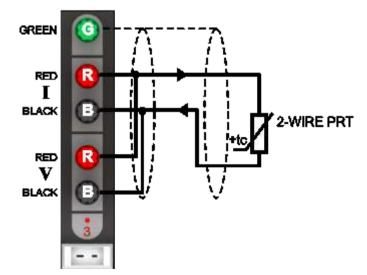
The connections to the PRT should be short (low resistance) in order to minimise the effect of lead resistance on the measurement. Alternatively, the connections can use remote sensing (using the 4-wire measurement capability of the milliK) to eliminate the effect of lead resistance completely. In this arrangement, the current and voltage sense connections are kept separate and are only joined close to the PRT:
