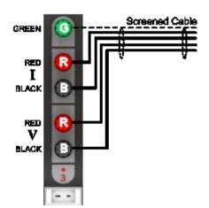
The screen should also be connected to the outer sheath of the PRT (if it is metal clad). The use of screened cables is more important when the milliK is used with thermistors, which have a higher resistance than PRTs or thermocouples.
